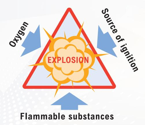
Effective ventilation reduces the chance of occurrence of them together and when selecting ventilation system, it should be ensured that they are suitable for the application and area served.
